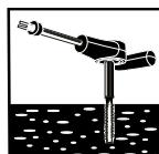
3a. TAP HOLE: Tap hole to the required depth using correct procedures (if unsure contact your dealer).
