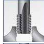
GAUGE the hole to recommended tolerance when required
