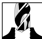
1. DRILL: Drill to clear out the damaged thread with drill size as specified on kit (if necessary).
