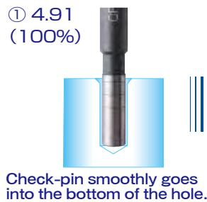
Check-pin smoothly goes into the bottom of the hole.
