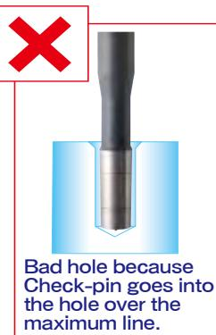
Bad hole because Check-pin goes into the hole over the maximum line.
