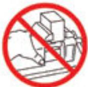
Do not hold the work piece or vice by hand, they must be clamped.
