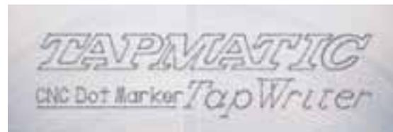
Mark logos using standard CAD/CAM software for the tool path.
