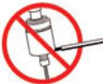
Do not lengthen the stop arm, it could break off.
