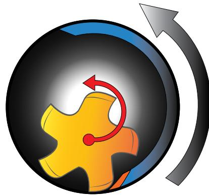
**It may be necessary to use more radial depth passes than shown on the chart (p.36) when cutting an unfavorable length-to-diameter ratio, coarse pitches, or hard materials.** When cutting a thread with two passes, cut approximately **65% of the thread on the first pass and 35 percent on the finish pass.** For three passes, use a **50/30/20** ratio. For four passes, use a **40/27/20/13** ratio. The idea is to equalize the side cutting pressure.
