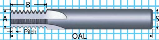
➤ All thread mills featured on this page can cut any larger size internal thread of same pitch
