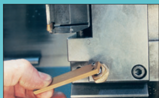
Short extensions aim easily with aiming tool (included).
