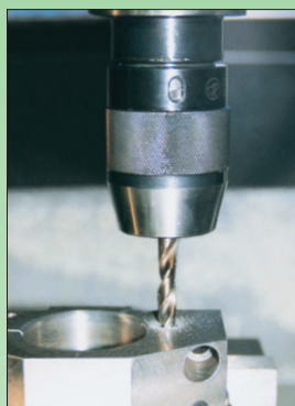
1 Drill coolant passage, leaving reaming allowance.
