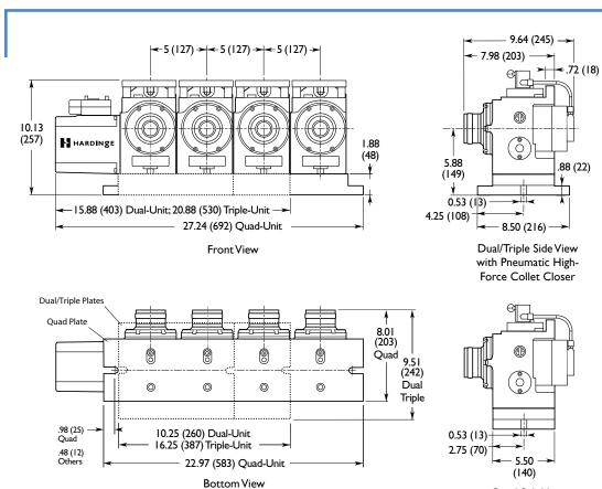
Quad Side View with Pneumatic High-Force Collet Closer
