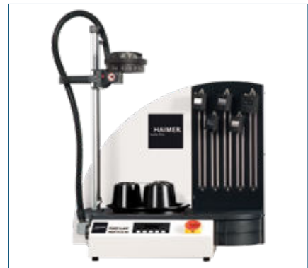
Power Clamp Profi Plus NG High powered shrink fit machine – Heating power 20 kW – For shrinking of tools from Ø 1/8"–2" (3–50 mm) – For HSS- and solid carbide tools – Big coil for Ø 1 1/2"–2" (40–50 mm) optional – Incl. rotary table and chuck support – Incl. tool tray – With craning boxes for accessories
