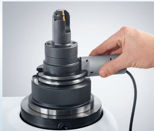
Manual positioning of the read/write head
