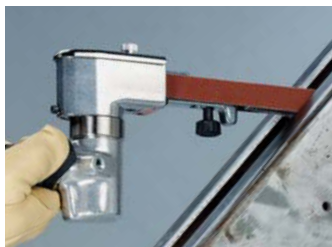
15400 Dynafire® III allows finishing and deburring in restricted areas.
