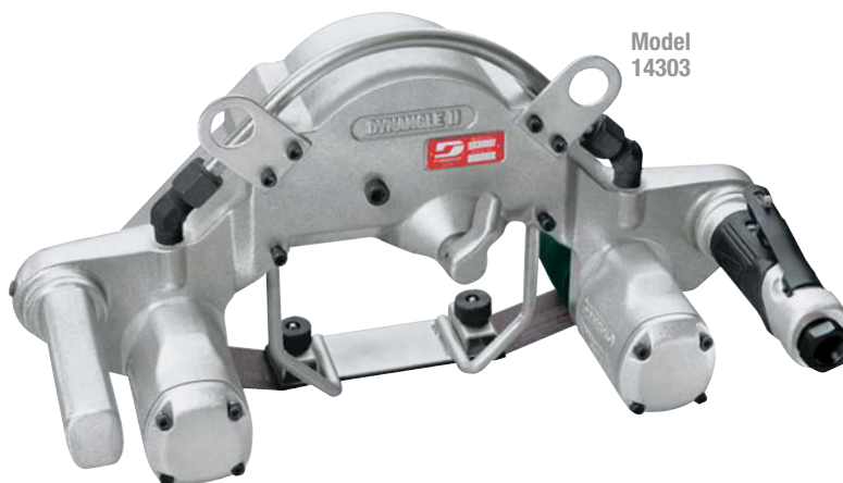
14300 Dynangle® II is utilized for "strap polishing" on a cylindrical stainless steel surface.
