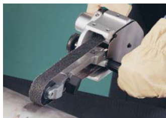
Model 11475 is ideal for grinding circumferential welds.
